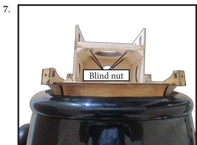
Attach the motor to the front of the electric motor box using four 5mm blind nut, four M4x20mm hex head bolts to secure the motor. Please see picture shown.
