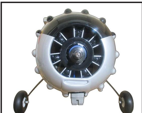
Attach the electric motor box to the firewall centered with the cross lines drawn on the electric motor box and firewall. Using M5x30mm to secure the motor box to the firewall. Please see pictures below.
