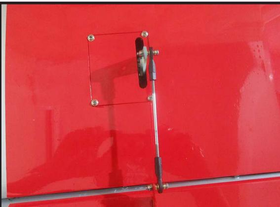
**INSTALLING THE FLAP PUSHROD**
