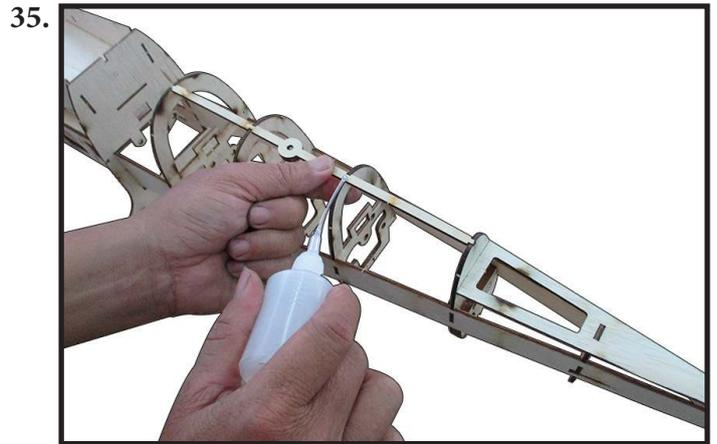
Locate and assemble F19 to fuselage by CA glue as photo shown (photo 36).
