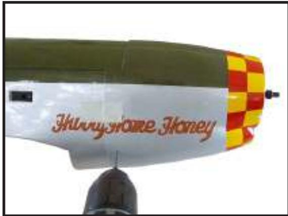
3) Tape a piece of card stock to the fuselage to indicate the location of the muffler, needle valve, and any other items that may require access when the cowl is mounted. Slide the cowl on the fuselage, and transfer these locations onto the cowl. Use a drill, rotary tool and sanding drum to make any cut-outs in the cowl before securing it to the fuselage.
