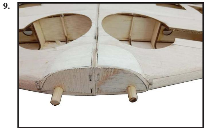
**\* Drill the holes for bolt at rear of wing.**
