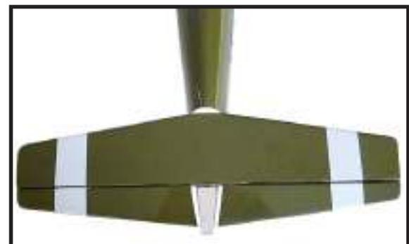
4) With the stabilizer held firmly in place, use a pen and draw lines onto the stabilizer where it and the fuselage sides meet. Do this on both the right and left sides and top and bottom of the stabilizer.
