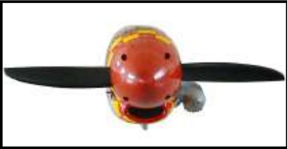
⚠ The propeller should not touch any part of the spinner cone. If it does, use a sharp modeling knife and carefully trim away the spinner cone where the propeller comes in contact with it.
