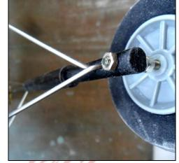
9. Being careful to not move the flap/slat servo, connect a short pushrod to the flap/slat servo's arm, and insert its other end into the quick-connector as shown below.
