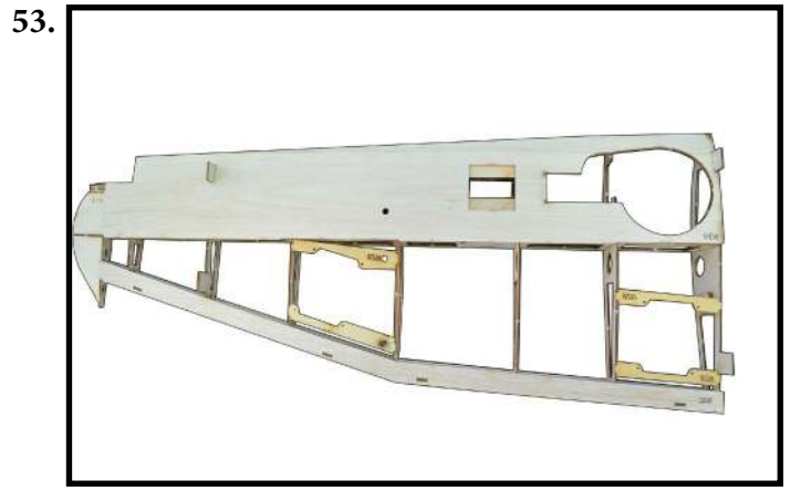
- Sheeting was finished.
