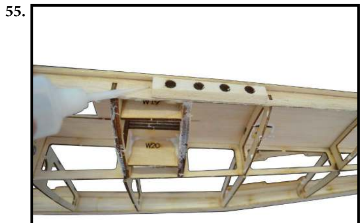
- Attach 6mm balsa block to leading edge at mount of gun as photo.
